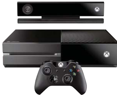
1. Microsoft's Xbox One employs a new Kinect 3D time-of-flight sensor.
