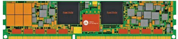
1. Diablo Technologies' Memory Channel Storage (MCS) plugs into a standard DIMM socket and implements the DDR3 protocol, but it has flash memory chips on board, not DRAM.
